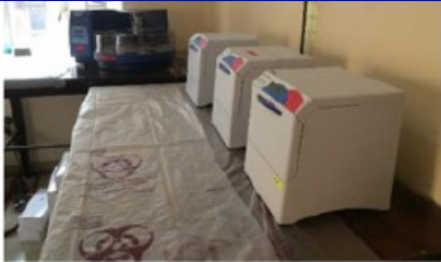
Room 2. The 96-well RNA extractor is in the center, 3 Bead Retrievers are on the right. Foil was placed over the window to deflect the heat of the sun
